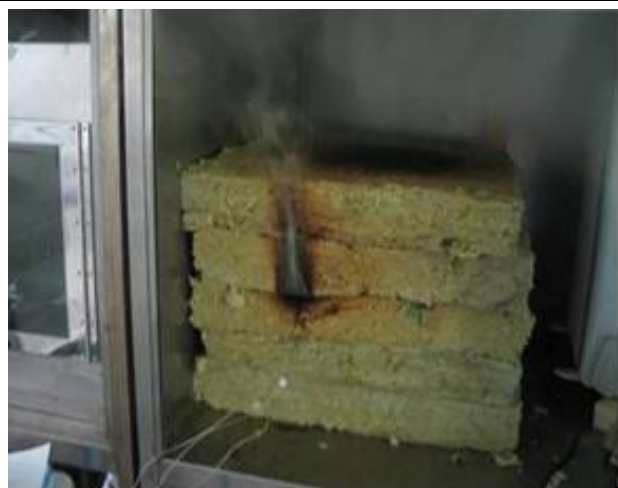
a) Test 4.6 : 5 hrs after the start of the test with boiled linseed oil . There was still some smoke from the test setup after 6 hrs, but after 7 hrs the smoke development has ceased.
