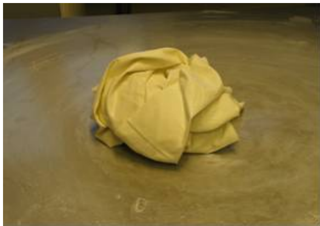
Test 4.4: One rag of area 1 m 2 with 100 ml Faxe wood floor oil before the test.
