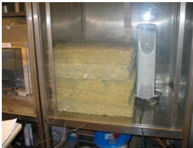
a) Experimental setup of Experimental Series 4 . Three 1 m 2 rags were placed in the centre of the 200 mm x 200 mm hole cut out in the 100 mm thick Rockwool mat in the middle mat (of the five mats).
