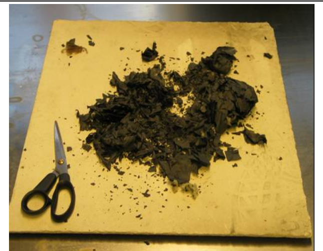
The highly charred residues of Test 1.8 in which four 500 mm x 500 mm large cotton rags (total of 1 \text{ m}^2 ) were evenly contaminated with a total of 1.0 dl of boiled linseed oil.
