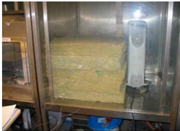
Faxe Wood Oil (loading: 100 ml/m 2 ) in 60 cm x 60 cm x 50 cm high block of Rockwool insulation.
