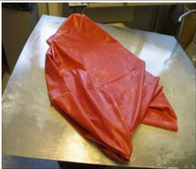
a) One of the three 1 m 2 rags after 100 ml boiled linseed oil had been evenly distributed in the rag.
