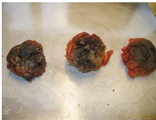
d) The rags after the test. They were rather burned in the contact surface between the rags but the opposite surface of the bottom and top rag were not burned. The rags were somewhat wet after the test.
