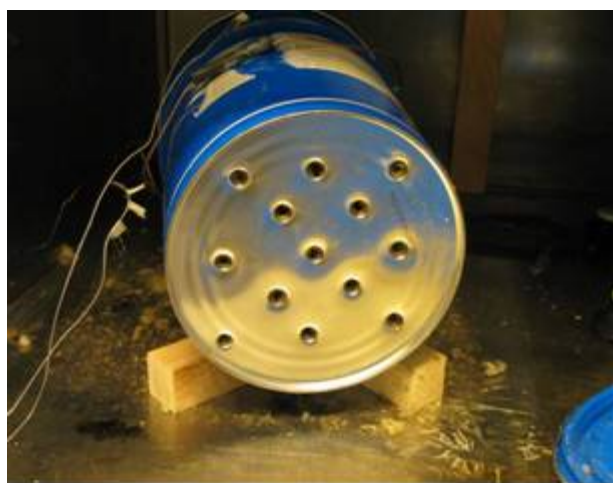
b) 13 holes were made in the bottom of the bucket and in the insulation above in order to improve the ventilation of the bucket.
