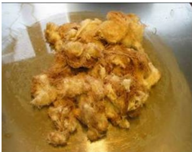
Test 3.2: The Twist rags supplied evenly with 0.3 litre Butinox wood oil.
