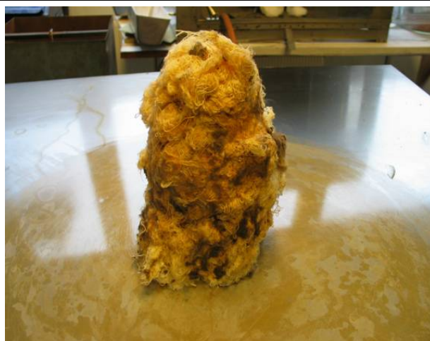
Test 3.1: 260 ml Owatrol oil (218 g) in three Twist rags of total weight 250 g. The three rags were rather agglutinated and slightly burned. The max. temperature achieved during the test was ~ 200 °C.
