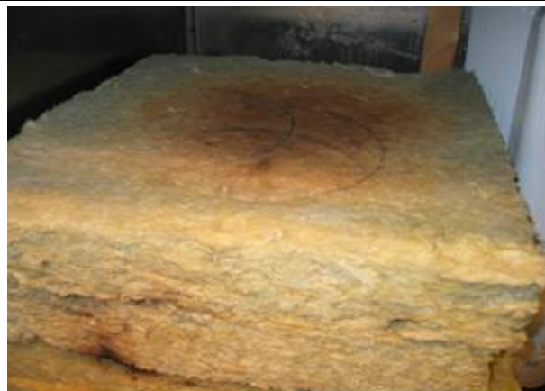
b) The test setup after the almost 30 hour long test. The upper mat is slightly brown due to the heat generation during the test.
