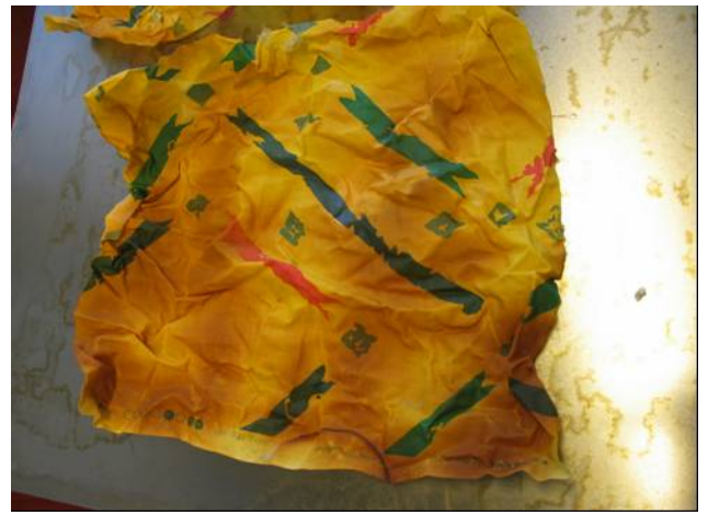
The picture shows the bottom rag in the bucket after the Test 1.6 was finished. Parts of the rag are somewhat brown and slightly burned (see the brown semicircle at the lower edge of the rag).
