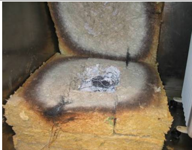
b) The test setup after the test when the two upper Rockwool mats were raised. The picture shows the cavity in which the three rags were placed after the 22 hours long test.
