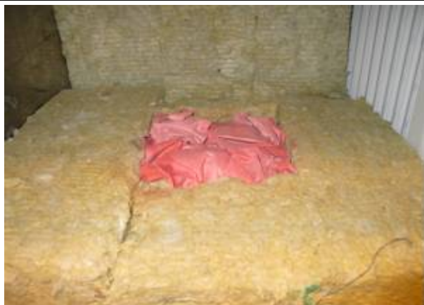
a) Test 4.5 : The three cotton rags with Faxe wood floor oil were placed into the cavity before as shown.
