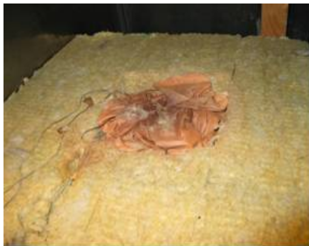
b) Test 4.4 : The three rags with Faxe Prestige wood oil (24 °C ambient temperature) after the test. The outer surface of the rags was slightly decolourized. The three rags were highly glued together in a massive clump.
