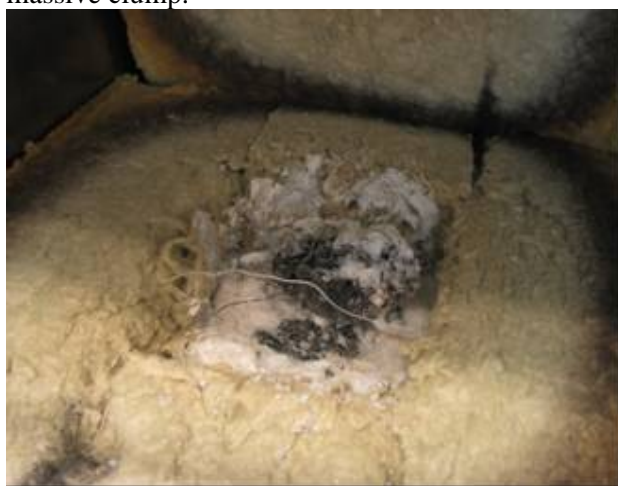
d) Test 4.6 : The residues of the 3 m 2 rags with Boiled Linseed oil at room temperature (i.e. 23 °C).
