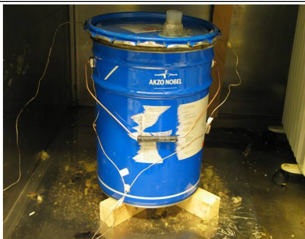
a) The test setup of Test 2.16 with 0.3 litre boiled linseed oil in 3 x 1 m 2 cotton rag and with increased ventilation of the rags.
