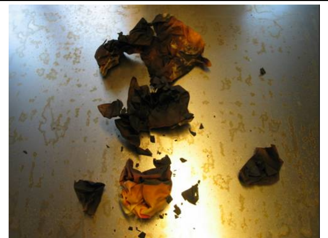
The three rags after Test 1.7. It appears that the rag in the middle (the rag located in the middle) is clearly most burned.
