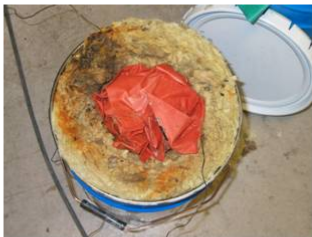
c) The three rags cotton rags filled the free space in the bucket completely.
