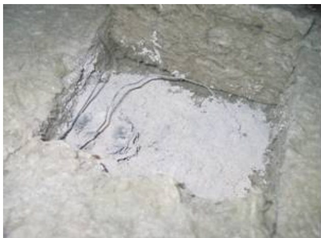
c) Test 4.5 : The residues of the 3 m 2 rags with Faxe Prestige wood oil elevated temperature (44 °C).
