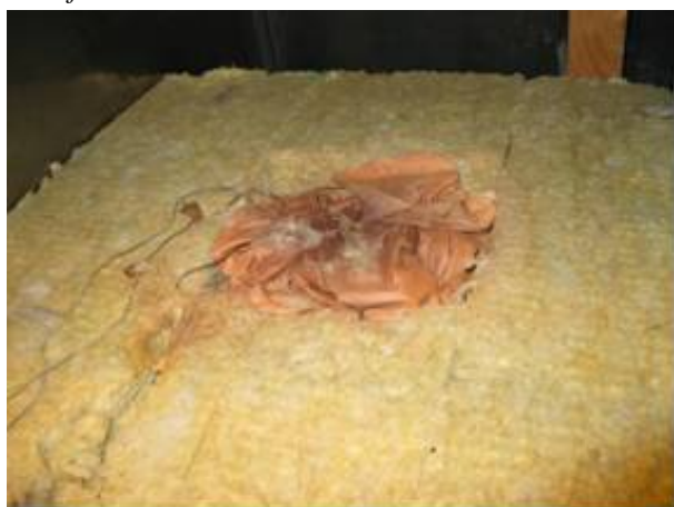
Test 4.4: One rag of area 1 m 2 with 100 ml Faxe wood floor oil before the test.
