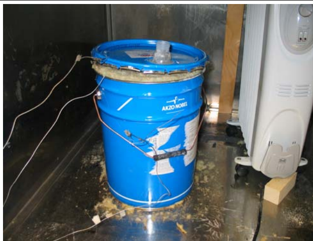
The test setup of experimental series 2, i.e. Test 2.1-2.14, where Twist rags were tested.
