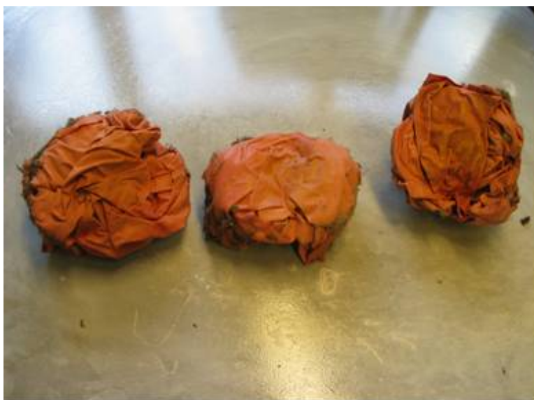
b) The cotton rags after the test. The rags were rather dry and slightly decolorized.
