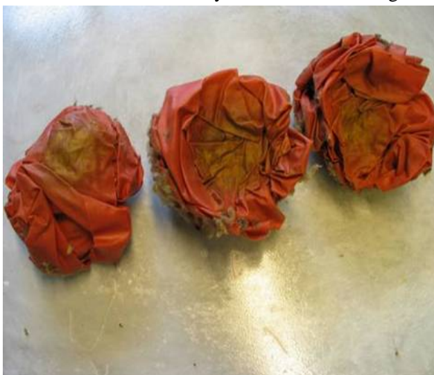
c) The three cotton rags after the 22 hrs long test with 0.3 litre boiled linseed oil .
