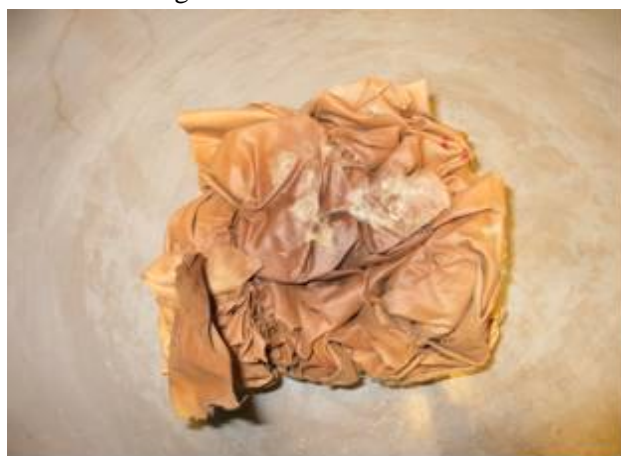
Faxe Wood Oil (loading: 100 ml/m 2 ) in 60 cm x 60 cm x 50 cm high block of Rockwool insulation.
