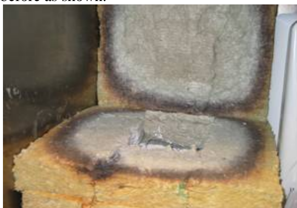
c) The fire damages of the Rockwool mat containing the cavity and mat above. The mats have become rather grey due to the fact that the cementing agent is lost due to the heat.
